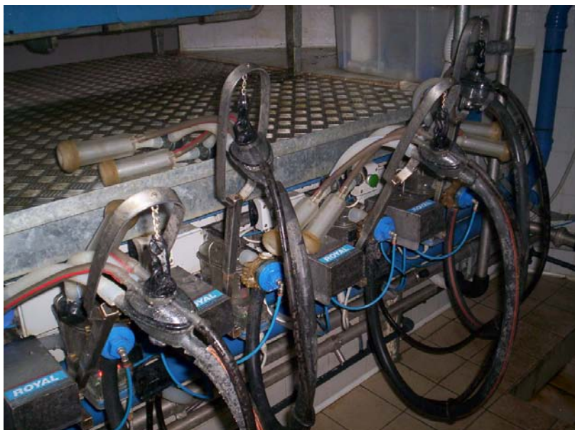
Figure 1. The innovative flow-based ACR installed on the milking parlour of the experimental farm of the University of Milan
